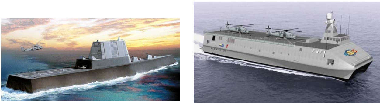
Figure 2 –Flat-Sided Ship Designs such as DDG 1000 (left) and War Fighter (right) are Ideal Candidates for Fabrication using Pultruded Flat Panels with Integral Joints
