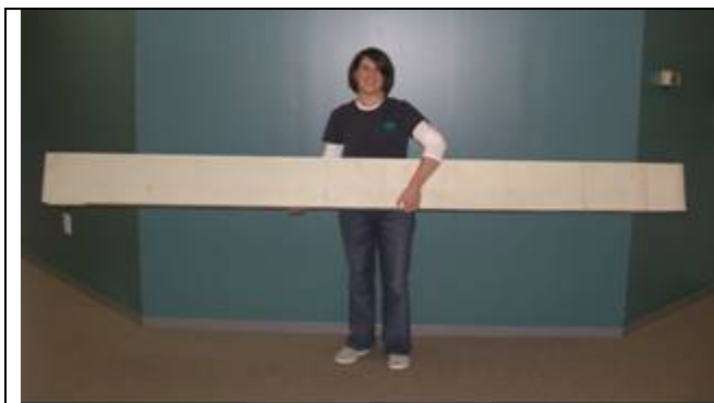
Figure 4a – Single Width of 10-Foot Wide Pultruded Panel Used as Basis for Ship Construction Cost Comparisons
