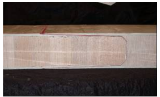
Figure 4b – Detail of Bonded Joint Connecting Parallel Sections of 10-Foot Wide Pultruded Ship Panel
